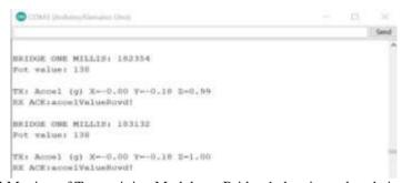
Fig. 1 Serial Monitor of Transmitting Module on Bridge 1 showing values being transmitted
